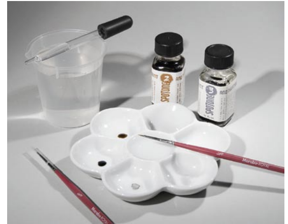
fig.2 Typical spotting tools include a large magnifying glass, a set of high-quality brushes, some blotting paper, a porcelain palette to mix and dilute the spotting dye, a cup of distilled water and an eyedropper.
